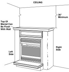
Figure 8-Mounting Clearances As Viewed From Front of Fireplace Shown with Optional Mantel
